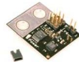
accelerometer, senses X, Y and Z acceleration
