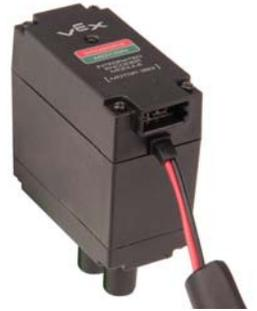
393 motor with encoder back, counts motor rotations, allows PID control
